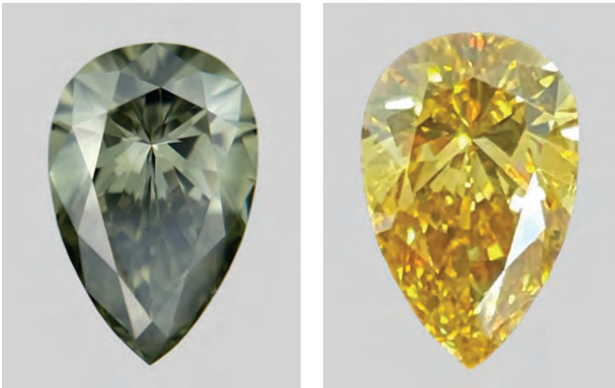
Figure 1. The dramatic colour change exhibited by a 0.87ct Chameleon diamond after heating from a candle.
