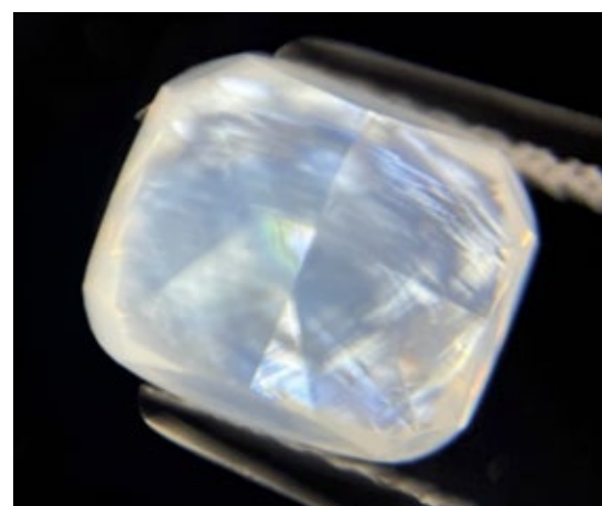
Figure 6. The birefringence pattern showing indications of plastic deformation.
