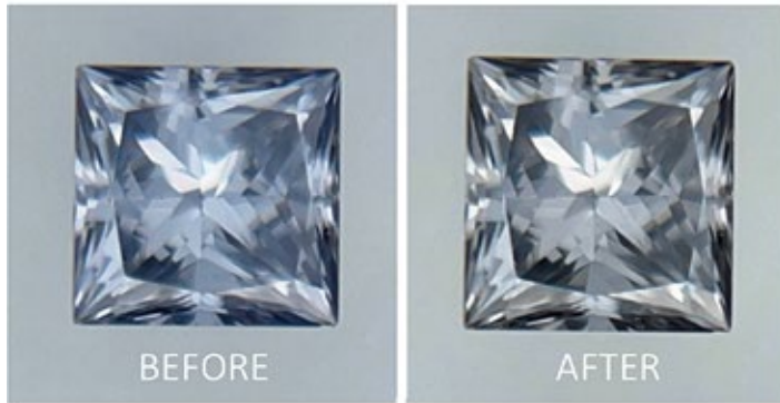
Figure 5. A 0.14ct Fancy Greyish-Violet diamond appears darker after illumination by SWUV light. The change is greater towards the blue end of the visible spectrum as seen in the before (red graph) and after (blue graph) absorption spectra of the diamond.
