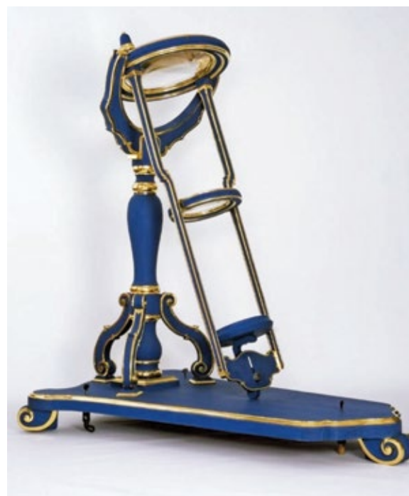
Figure 3. The Lens of the Royal Palace. This instrument's primary lens had a diameter of 89cm and thus a surface area nearly four times larger than the Bregans Lens. 1 Image by Michael Lange, courtesy of the Mathematics-Physics Department of the Dresden State Art Collections; ©Staatliche Kunstsammlungen Dresden/Mathematisch-Physikalischer Salon and reproduced with permission.
