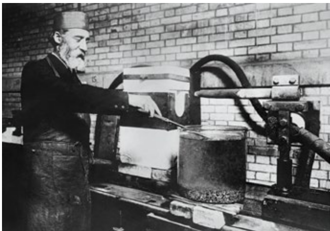
Figure 8. Henri Moissan quenching molten cast iron (alongside the electric arc furnace he invented). Image from Archive Pics, Alamy stock photo.
